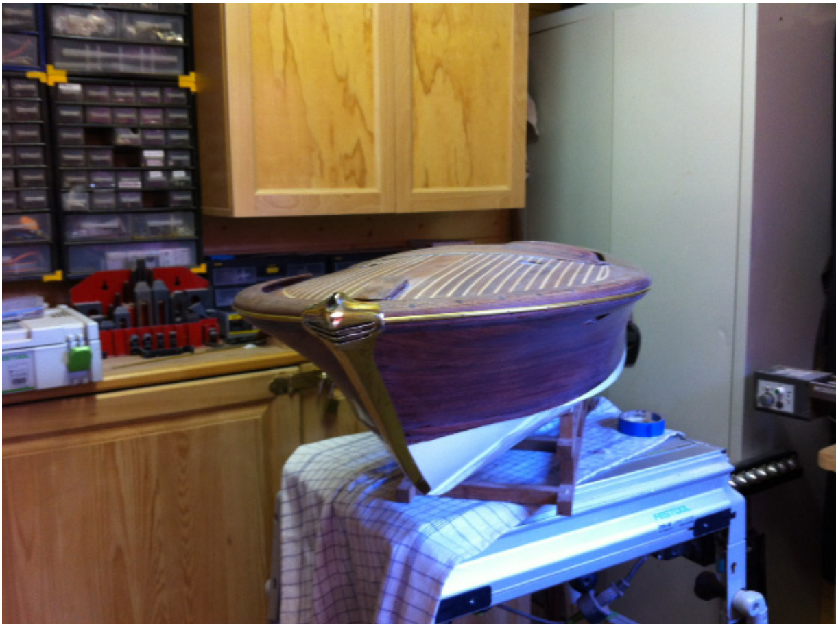
Painted surfaces are sanded for the 5th time and the tail plate, nose and side moldings are mounted and adjusted before chrome plating.
