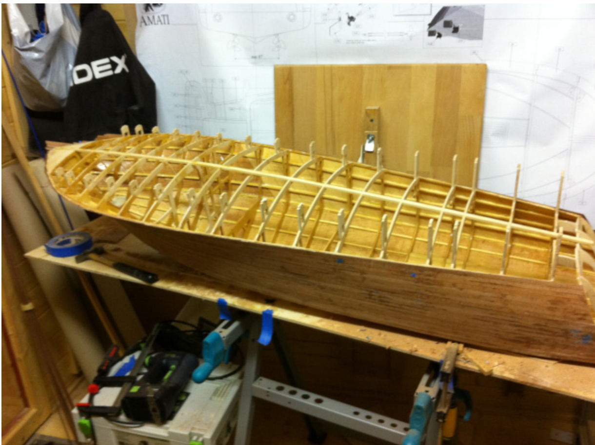
Sides and front of boat now covered with mahogany moldings.
