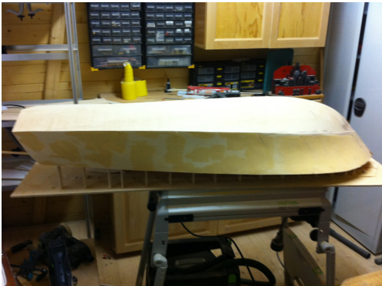
Bottom and sides finished and filled for the first time.
