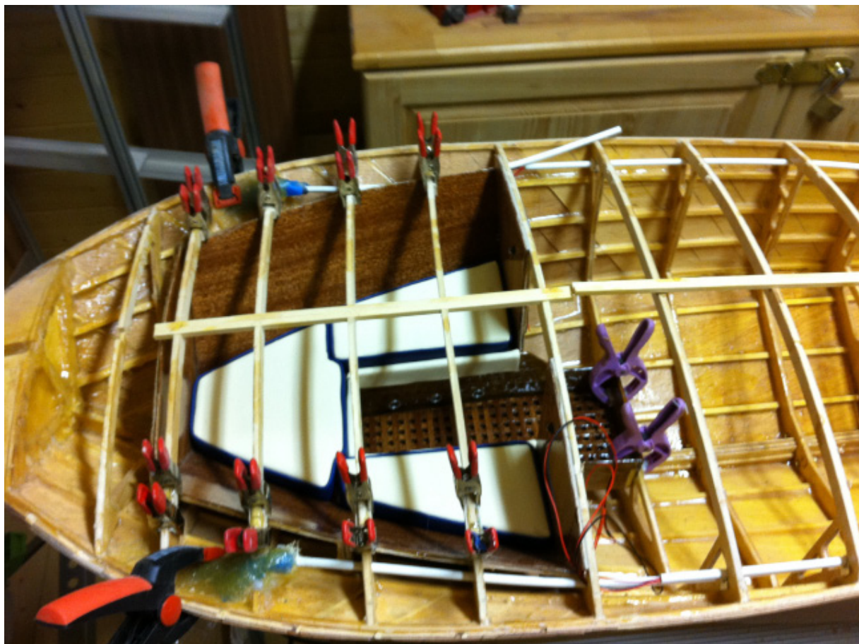
Cushion plates and sides in the cabin are installed after treatment with epoxy PERMAKOTE, the loose cushions and grate at the bottom are removed before further work.
