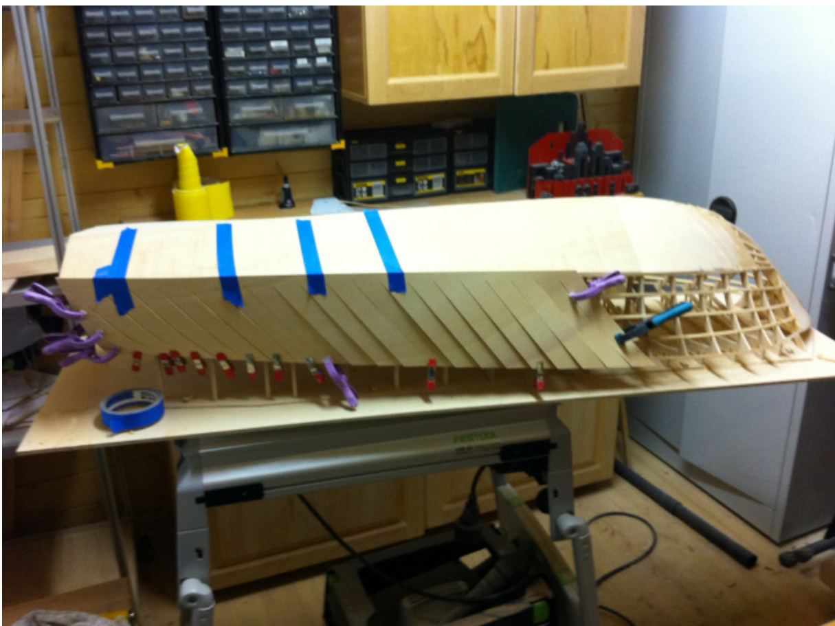
Adaptation of side fairing that is slotted open to more easily make it follow the lines of the hull
