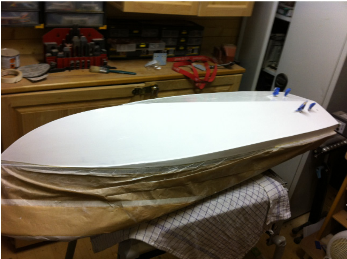
Bottom is now finished painted with Epifanes Polyurethane paint.
