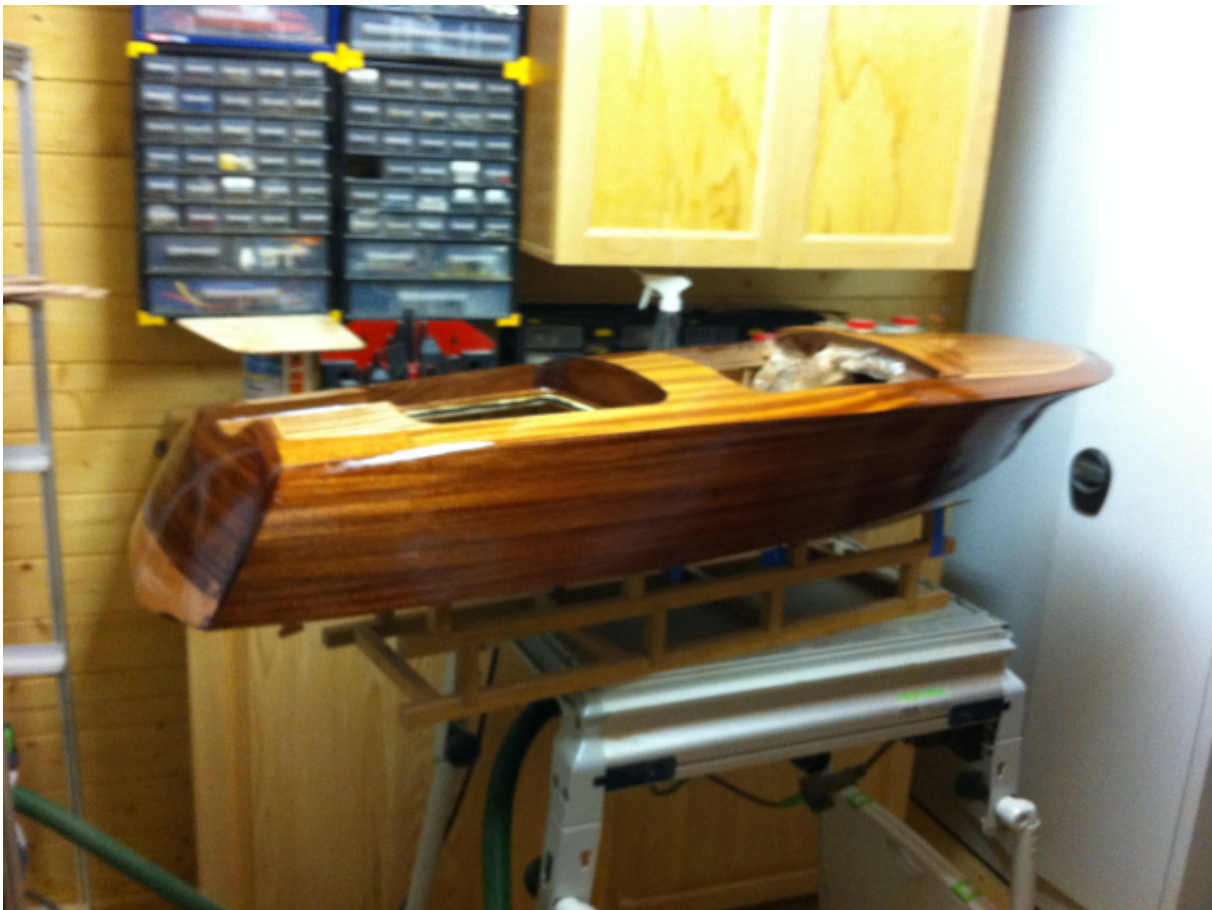
Boat deck etc fitted and the boat has had the first 4 coats of varnish.
