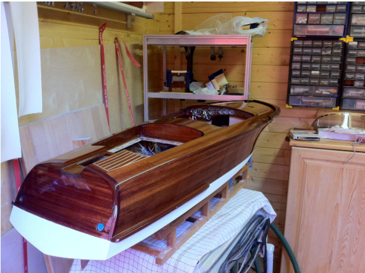
Paint work is now complete, 26 layers of paint give an unusually nice surface, instruments and steering wheel mounted.
