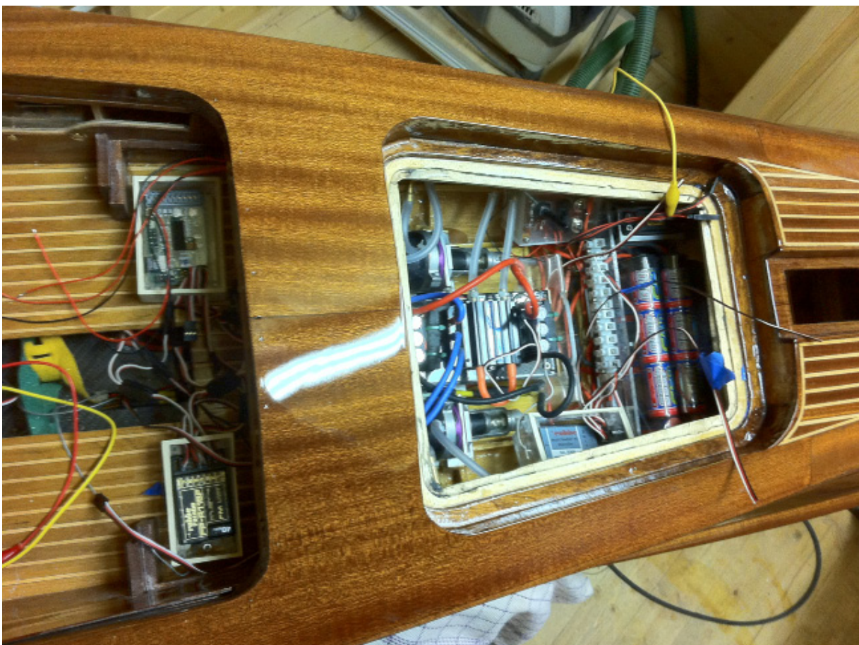
Before mounting fittings and covering edges etc. with artificial leather, the electronics are mounted and tested.
