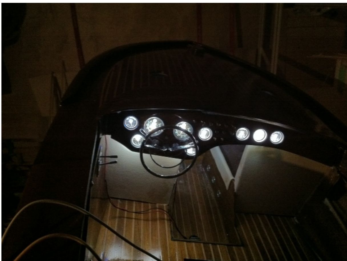
Test of light in instruments, right and throttle, mounted on mahogany side plate which is treated with epoxy PERMAKOTE on both sides.
