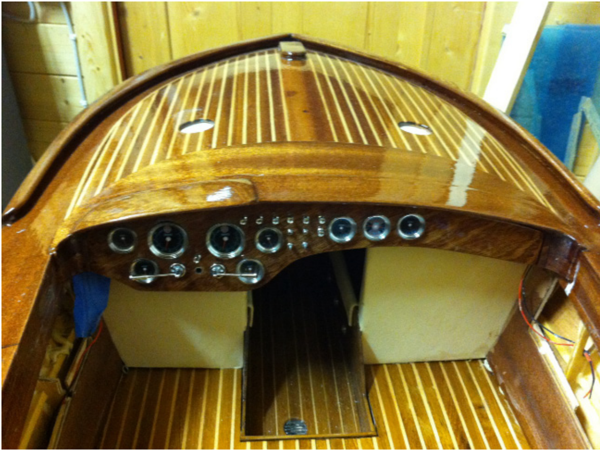
Test fitting of instruments, openings in the sides are for servos to control the steering wheel and throttle movements, the deck is clad with oak and birch strips.
