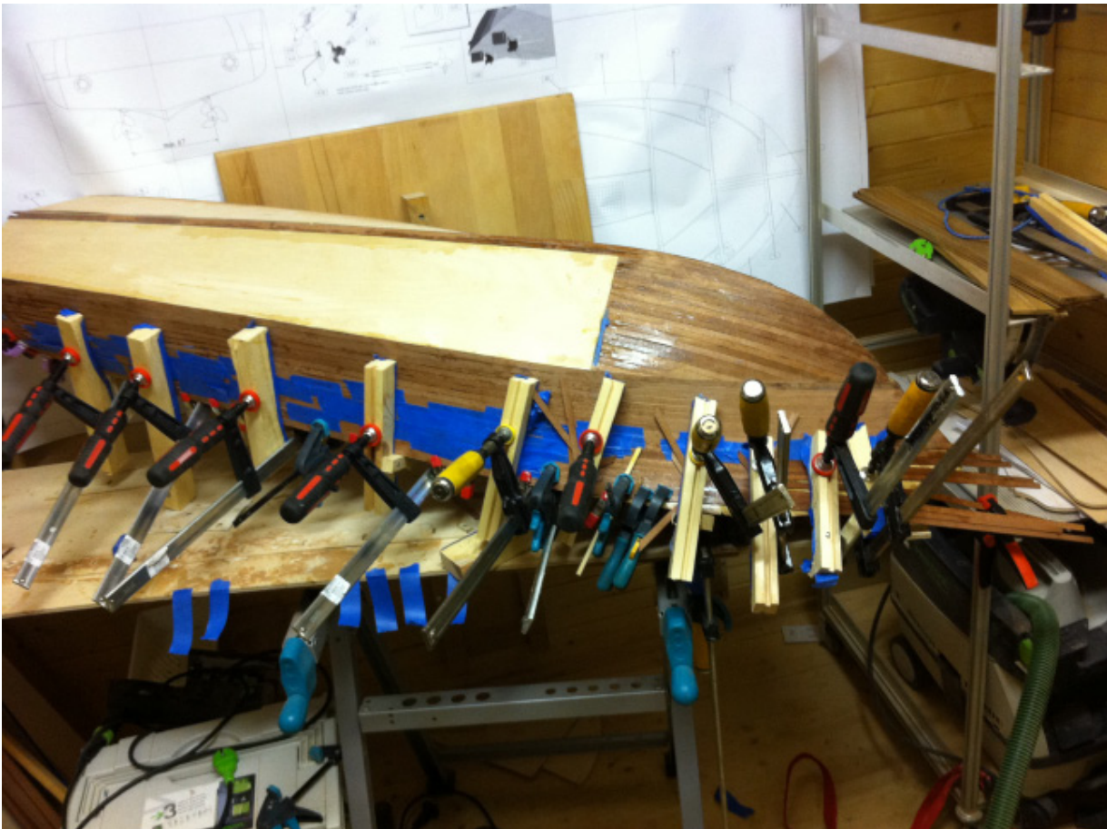
Cladding with mahogany moldings, masking tape is used to prevent “press blocks” from being glued to mahogany moldings. Epoxy of the WEST SYSTEM brand is used for gluing.
